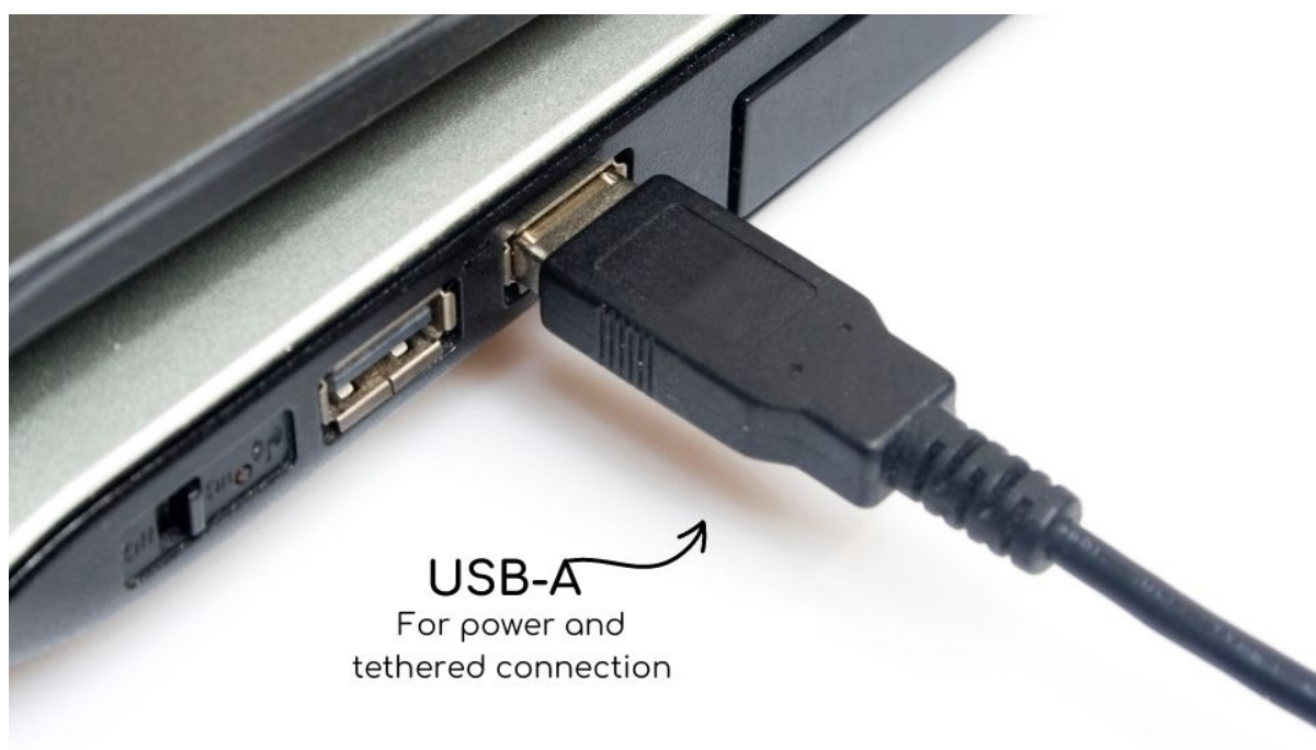
Fig. 2.5: USB Connection to the PC/Laptop
