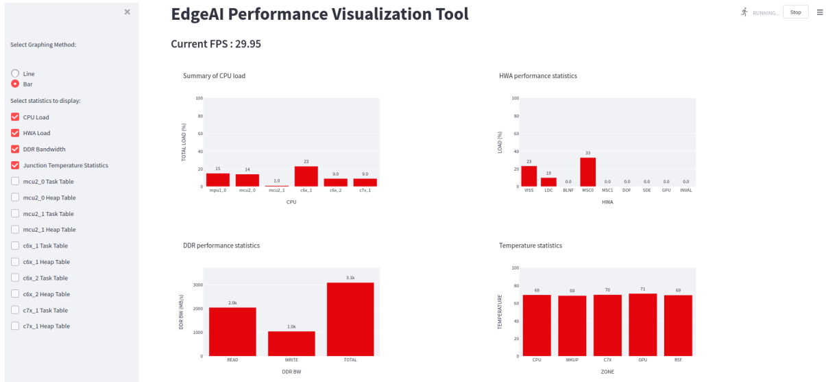
Fig. 5.15: Performance visualizer dashboard showing CPU and HWA loading, DDR bandwidth, Junction Temperatures and the FPS obtained
